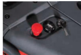
Key-switch, emergency switch and battery discharge indicator.
