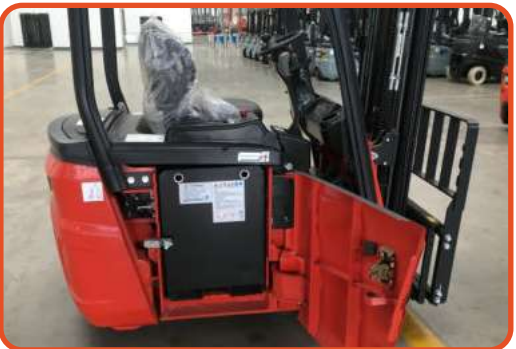
■ Battery compartment with fork pockets for 16N
