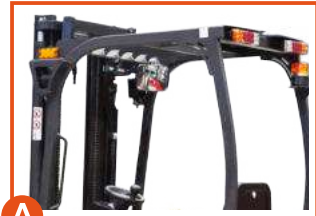
A Front LED Lights, Steering lights, Rear Combination Lights, Warning light standard, safe to work in dark environment such as containers or in the night.
