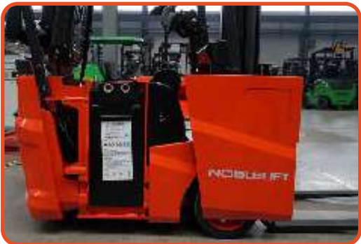
■ Battery compartment with rollers for 08-12N
