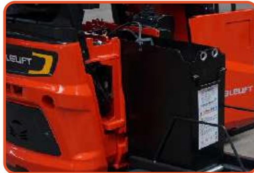
■ Battery compartment with rollers for 08-12N
