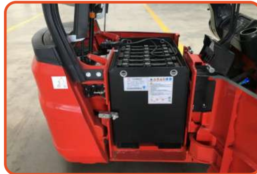
■ Battery compartment with fork pockets for 16N
